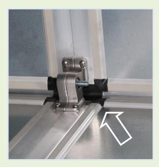
The two gaskets, GS-20 and G002, create a *unique and continuous element* along the whole edge of the panel, thus determine a *smooth and radius area inside the unit* so the AHU *meets the Hygienic standard requirements according to DIN 1946 Part 4*, ie with the absence of internal protruding objects.
